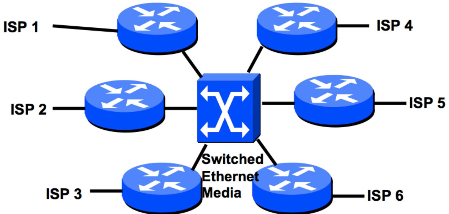
**Each router represents a border router in a different autonomous system (ISP)**
